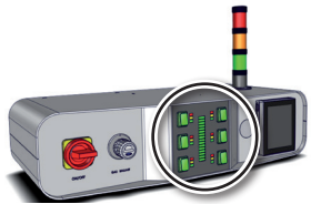
Switch on individual vacuum pump
